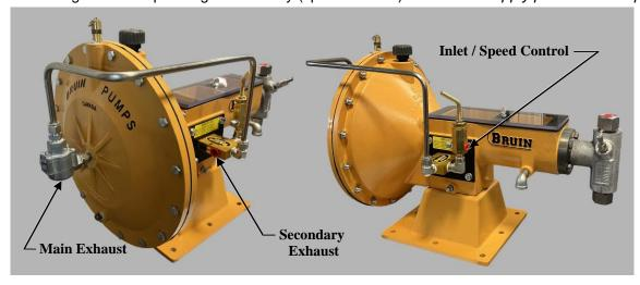
The BR5000 Quick Exhaust Conversion Kit (BB-0037QE-CONV) allows for a BR5000 with a Master Valve Assembly to be converted into a Quick Exhaust setup. An alternate high volume microswitch option (BA5100-02H) is available allowing for an increased maximum stroke speed.
